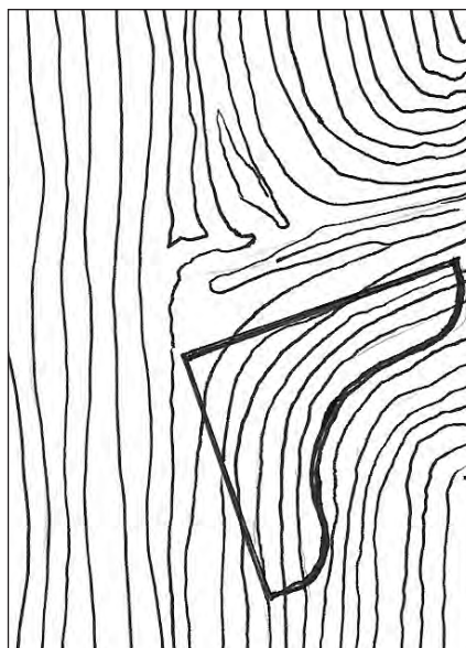
The drawing shows the placing of a template over a piece of timber with ideal grain pattern prior to cutting.
