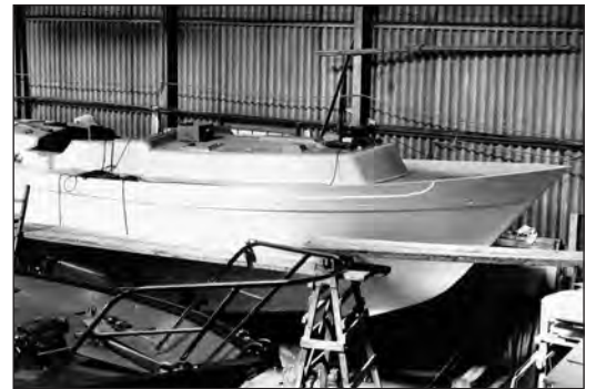
Photos above and below: Halberdier 36 mouldings ready for fit-out, circa. 1968 at Swanwick. Photo from David Moody collection.
