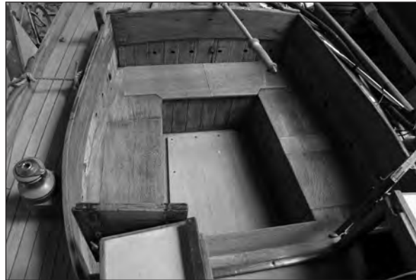
View of Vindilis' cockpit. Note the side cockpit combings. This allows for good visibility forward. Photo from David Moody collection.
