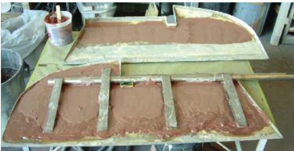
The two halves cleaned out and starting the rebuild
