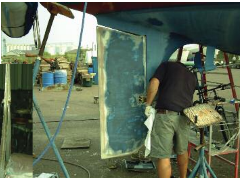
Edges smoothed and rudder refitted
