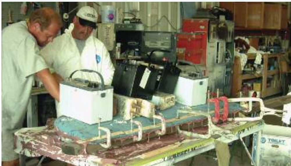
Joined, weighted down and clamped
