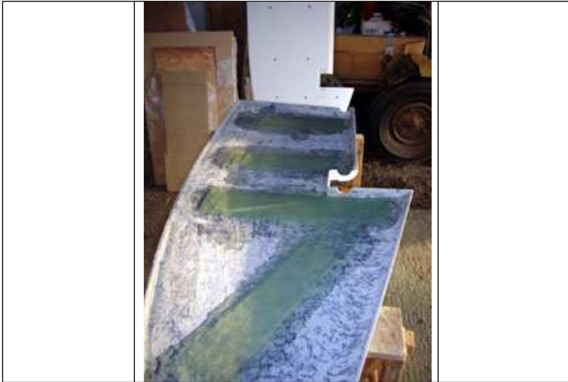
Nuts were welded onto each side of the rudder plates in line with the holes.
