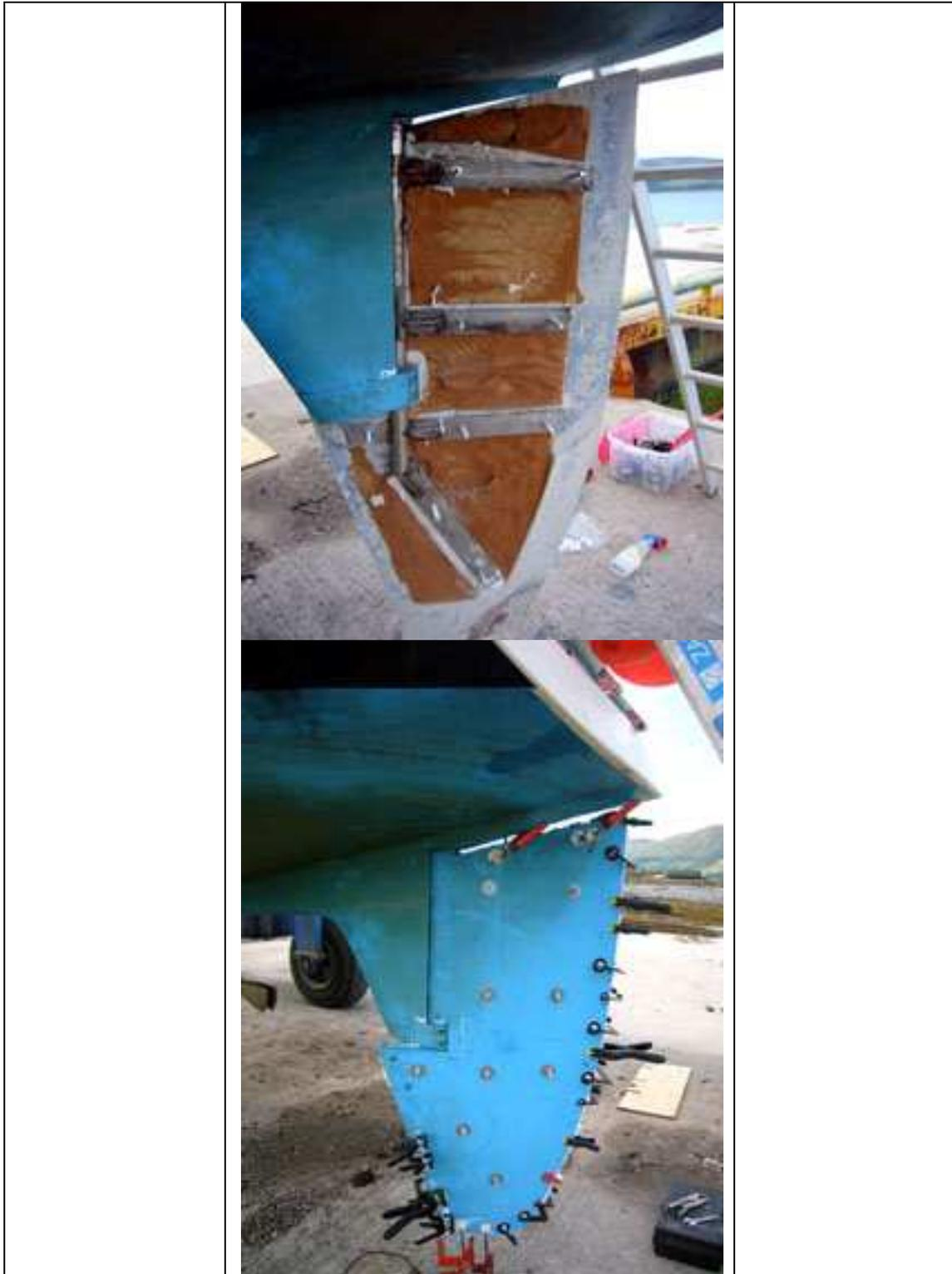
On lift out at the end of the season, the rudder was removed by first unbolting the steering mechanism. At this stage I discovered that the “earthing” cable which should have been attached to the rudder stock was broken. The rivet heads on the lower rudder bearing shoe were drilled off and the rivets knocked out. The heads of the slotted screws holding the lower bearing were in a poor condition, possibly electrolysis due to the rudder having no direct connection to the sacrificial anode.
