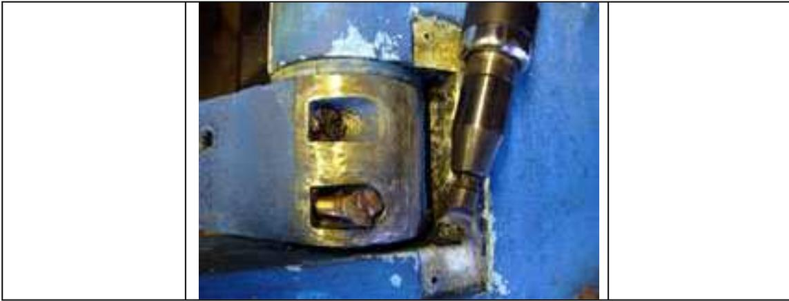
An impact screwdriver was needed to loosen these screws but the heads of two had to be drilled out. All the screw threads were in perfect condition. This posed an additional problem as it proved impossible to source replacements - the screw threads were found to be the old British Standard Whitworth and no longer available. However a length silicone bronze rod was purchased and a friend who had access to a lathe kindly machined new ones. A drill, made from a piece of steel tube,
