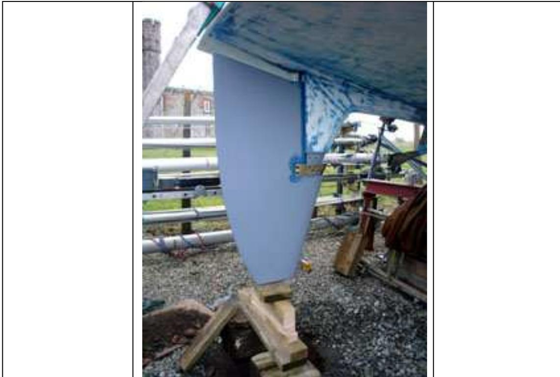
The whole assembly was then lowered slightly, to allow sealant to be applied to the inside of the shoe, before being raised once more and the new rivets inserted.
