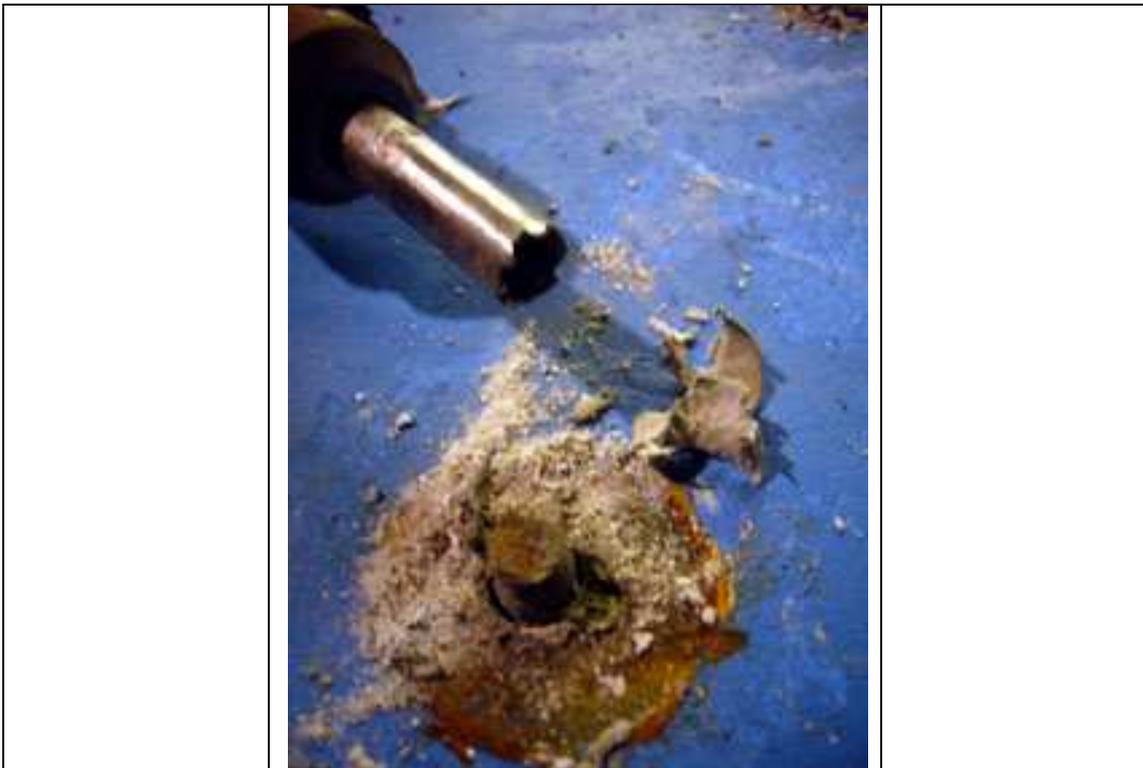
had to be used to release the temporary bolts holding the two halves of the rudder together, before they could be removed and the rudder split, with great difficulty, using an old paint scraper and a hammer. The polyurethane glue had done a superb job and there was little evidence of water ingress. (P1030321)
