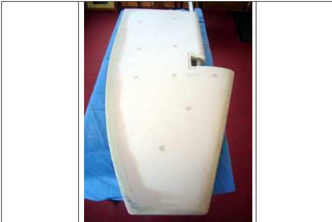
The rudder was then given four coats of epoxy paint prior to refitting.
