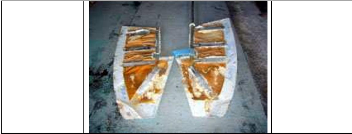
The foam and binder were chipped out of both shells.
