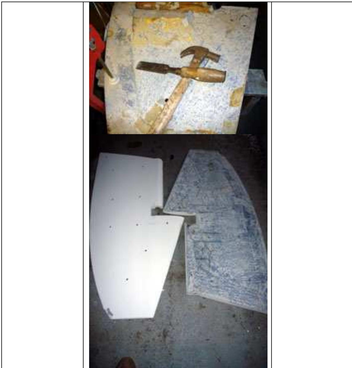
Glass fibre mat and resin was laid up in strips to thicken each shell so that the existing holes, drilled for the temporary repair, could be countersunk to receive screws in place of the bolts.
