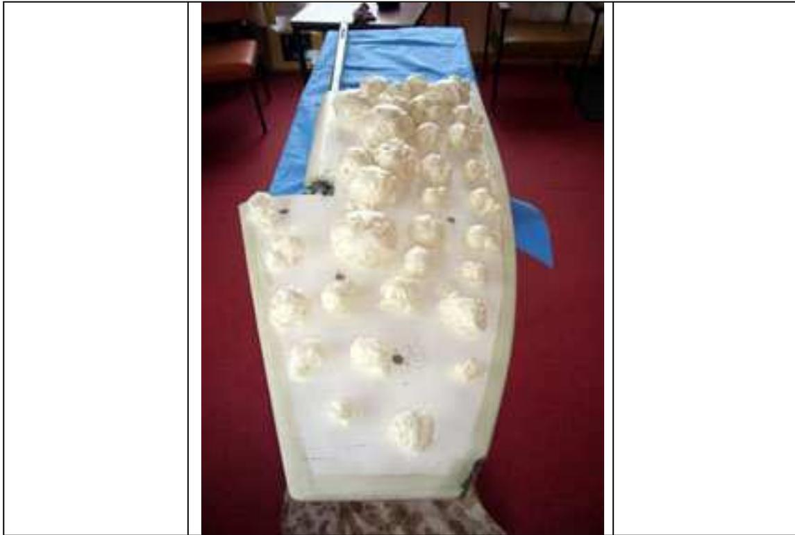
The injection holes were countersunk to give an increased surface area for the final filling and fairing.
