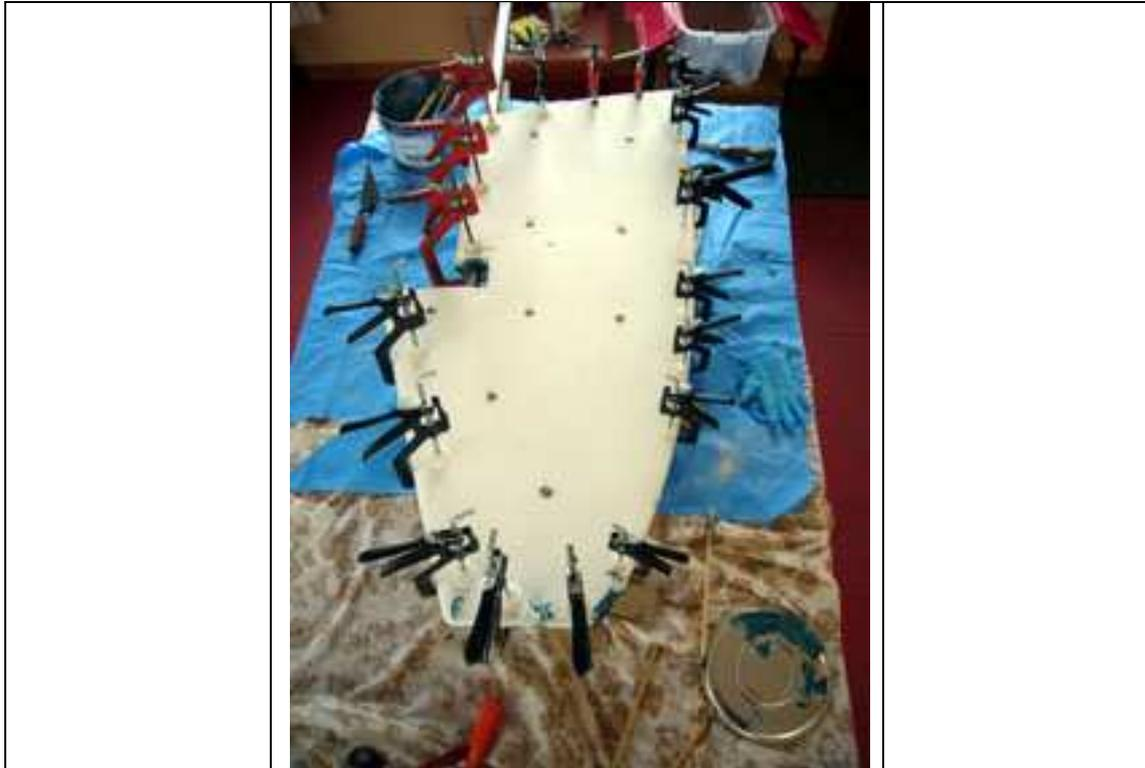
Three layers of glass tape were laid up around the edges, filled and faired. Numerous holes were then drilled into the voids and expanding foam injected in and allowed to expand and set before cutting away the excess.
