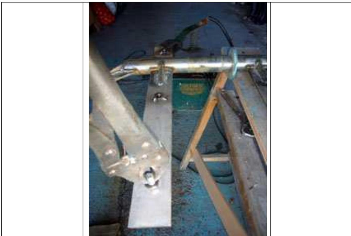
The rudder was then dry assembled to determine the correct length of screw needed for each fastening and the size pencilled beside each hole. The countersunk screws were cut to length and one half of the shell was fastened to the stock. Polyester filler paste was trowelled into the shell beneath the plates and round the rudder edges and stock.
