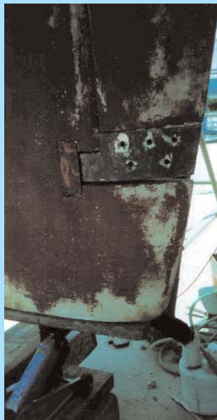
Above left: Lowered rudder shafts showing oxide deposits
