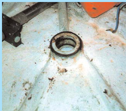
Existing rudder shaft hub with o-rings
