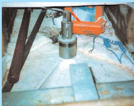
Extended rudder tube and additional o-rings prior to glassing to hull
